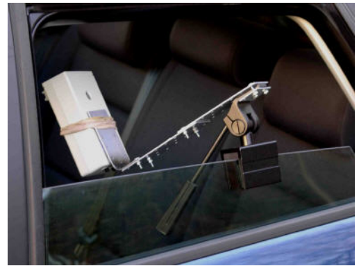
Figure 4. The detector mounted for a survey [Photo: Ralph Cordey]
