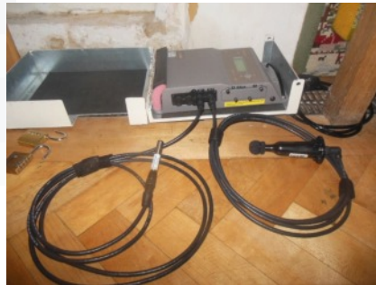
The RRMP SM3 detector and microphones preparing for set-up at All Saints, Wrabness
